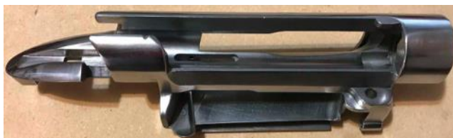
According to The American Krag Rifle and Carbine by Joe Poyer, a Model 1898 receiver made in 1900 required over one hundred twenty separate machining operations.
